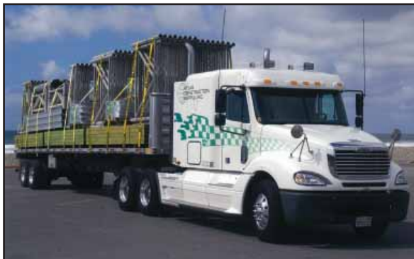
*One Semi-truck can carry up to 10,000 Ft 2 of shoring equipment for up to 12" deck.
